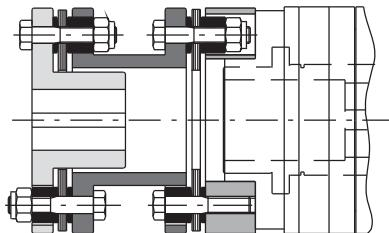
Model DSR/F/AP with single flexing disc coupling GTR-S, for applications where torsional rigidity is required and without the ability to accommodate radial misalignment.
