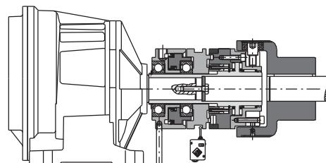
Model **DSR/F/AP** with Compact elastic coupling **GEC** for coaxial shaft transmission.
